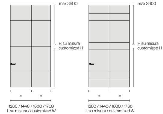
EN The panel is available with full-length mirror or with decorative horizontal and vertical crosspieces. The aluminium frame of Radius is available in aluminium, brown and 46 Ecoloursystem finishings. The double-sided door panel cladding is available in glossy, mat, reflex, sahara, diamante and mirror lacquered glass or in Litech, sahara and taiga essence, fabric or synthetic leather, for a total of 161 finishings.
