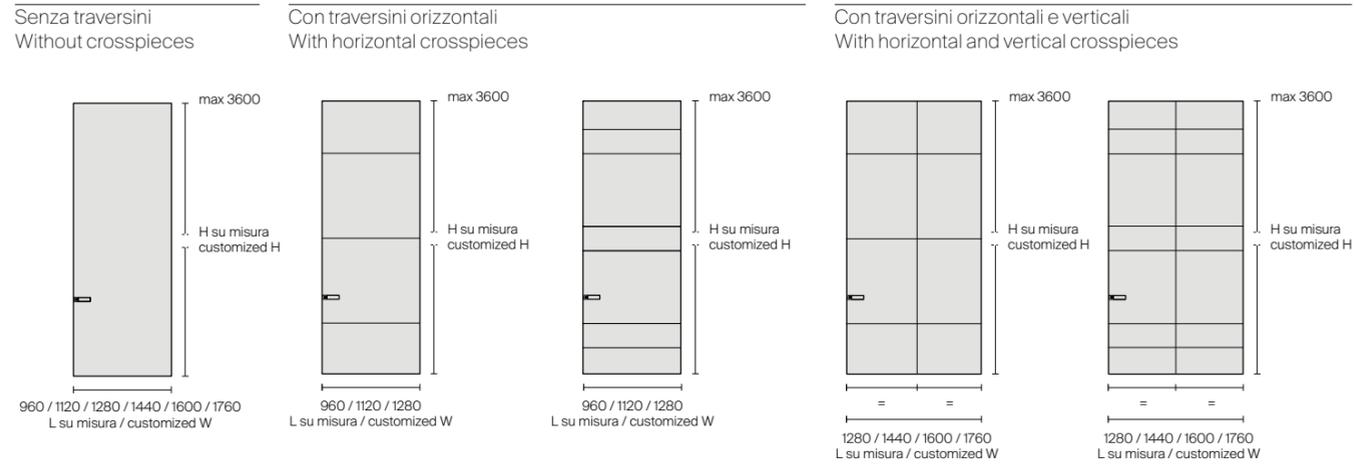
EN The panel is available with full-length mirror or with decorative horizontal and vertical crosspieces. The aluminium frame of Radius is available in aluminium, brown and 46 Ecolorsystem finishings. The double-sided door panel cladding is available in glossy, mat, reflex, sahara, diamante and mirror lacquered glass or in Litech, sahara and taiga essence, fabric or synthetic leather, for a total of 161 finishings.
