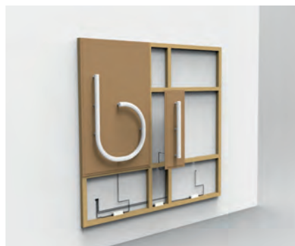
3. Attachment of panel b and connection of panel i to the power source.
