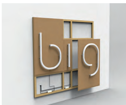
4. Attachment of panel i and connection of panel g to the power source.
