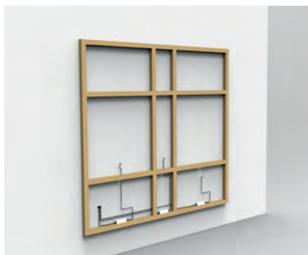
1. Creation of the supporting frame to provide space for power connections for the individual letters.
