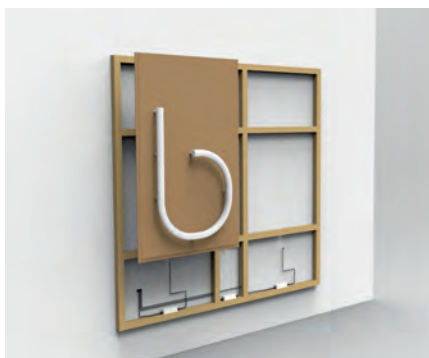
2. Connection of panel b to power source.
